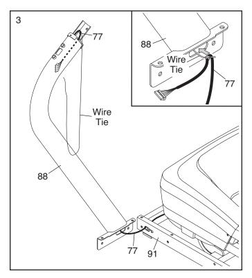
Hold the Left Upright (88) against the Base (91). Be careful not to pinch the Upright Wire (77) or the Ground Wire (90). Insert two 3/8" x 2 3/4" Patch Bolts (7) and two 3/8" x 1 1/4" Patch Bolts (8) with two 3/8" Star Washers (13) into the Left Upright.
